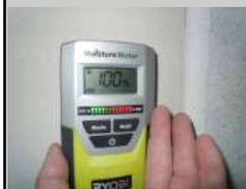
This is one type of meter we use. It reads moisture content.
